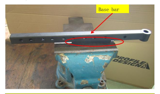
Clamp the base bar on the bench vise, make sure the base bar is clamped firmly, as the picture shows.
