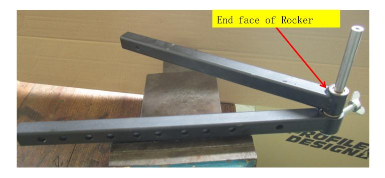
Insert the rocker into axle shaft, make the end face of rocker be parallel with the sectional face of axle shaft.
