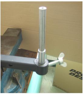
Install the axle shaft on the base bar and then fastened by the screw firmly.
