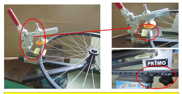
Put the wheel rim without tire on the axle shaft vertically, make sure the rim on the lower clamp pad, and then fastened the clamp assembly by screws.
