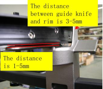
According to the OD of the rim, adjust the position of large tire guide and then fasten the screws at the bottom. Please refer to right picture.
