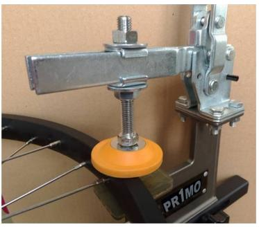
According to the width of rim, and then adjust the nut of upper clamp to make the rim fastened with the clamp, finally fasten the nut on the clamp.
