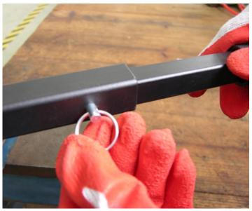
Insert the lengthening bar into rocker, and adjust the position according to the force of assembly, fianlly, fastened by the quick bolt firmly.
